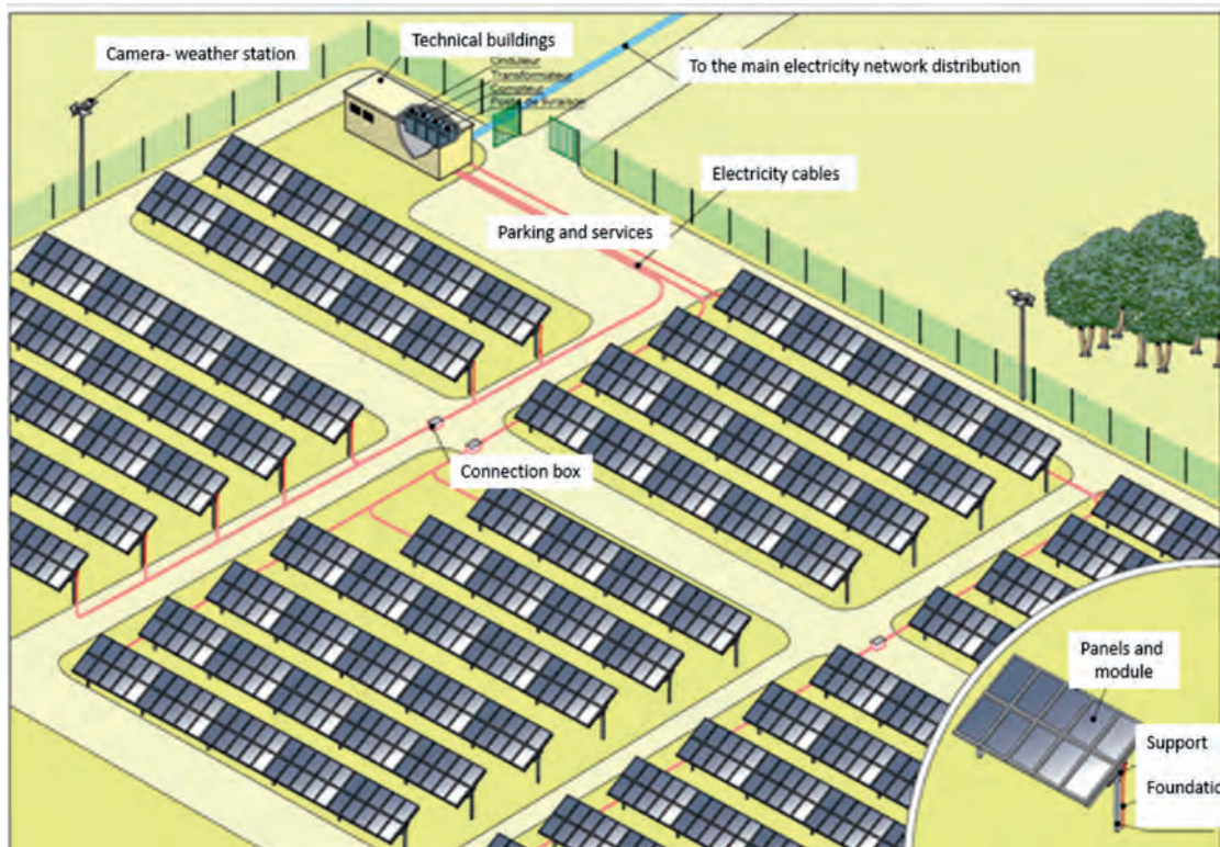
Fig. 2. Photovoltaic central, photovoltaic panel, cables, technical buildings, connection to the main energy gride, etc. MEDTL, 2011
